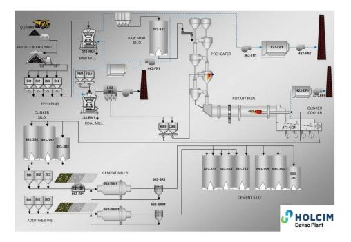
Note: dashed lines indicate production steps that do not necessarily apply to this cement
