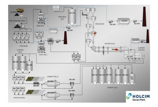
Note: dashed lines indicate production steps that do not necessarily apply to this cement
